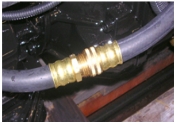
Separate Exhaust Manifold Drains
