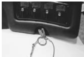
Figure 2-7. Stop Switch Lanyard
