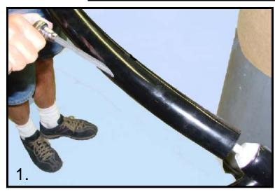
Align protruding ½" bolt into tapered mount. Insert special allen wrench included with tower into opening located on outside radius of tow bar. Tighten bolt about halfway down using 3/8" socket with ratchet wrench.
