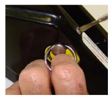
4. Begin screwing Ball Plunger counter clockwise a quarter turn at a time while pulling on Retainer Ring.
