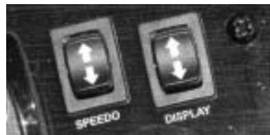
Figure 2-4. Speedometer Calibrate and Display Selection Switches
