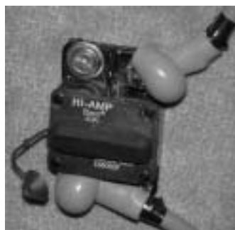
Figure 4-4. Main Circuit Breaker
