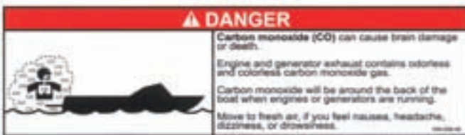
Figure 1-5. Carbon Monoxide Hazards
