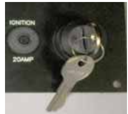
Figure 2-15. Remote Ignition Key Switch
