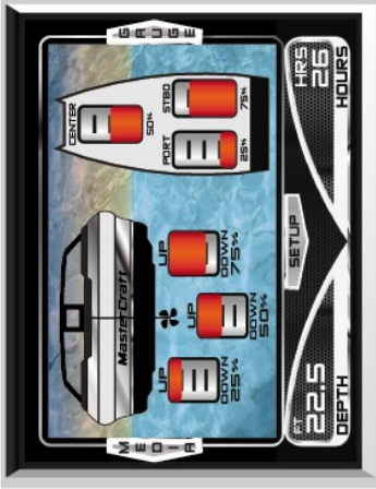
BALLAST/TRIM MAIN SCREEN
