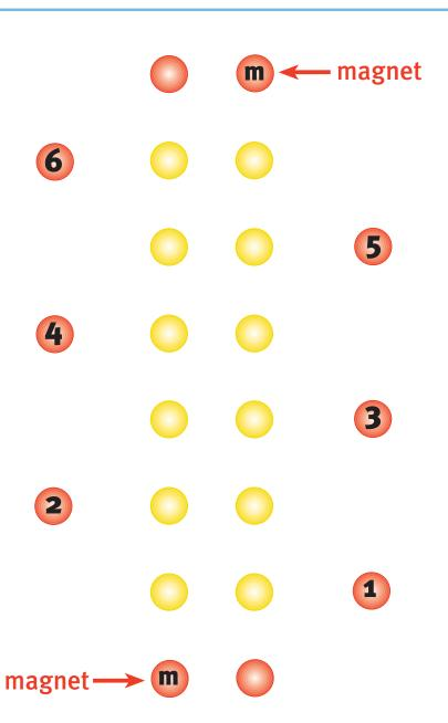
When running with one "Smart Timer" magnet sensor on passenger side, only two magnets are required as shown.
